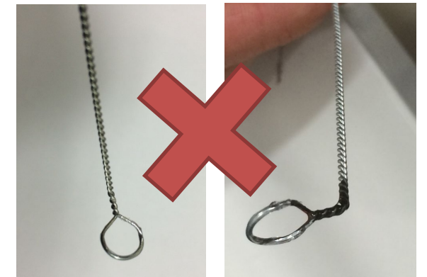
S/S wire loop - corrosion
