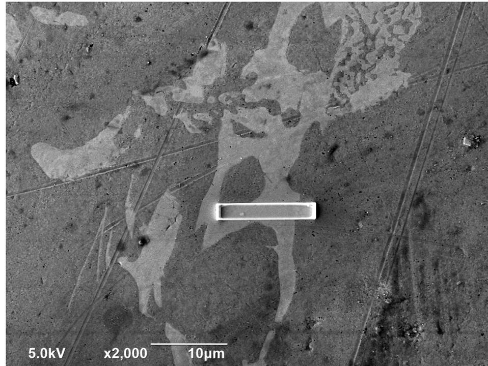
**i) Electron beam-assisted Pt deposition (Pt edep)**
