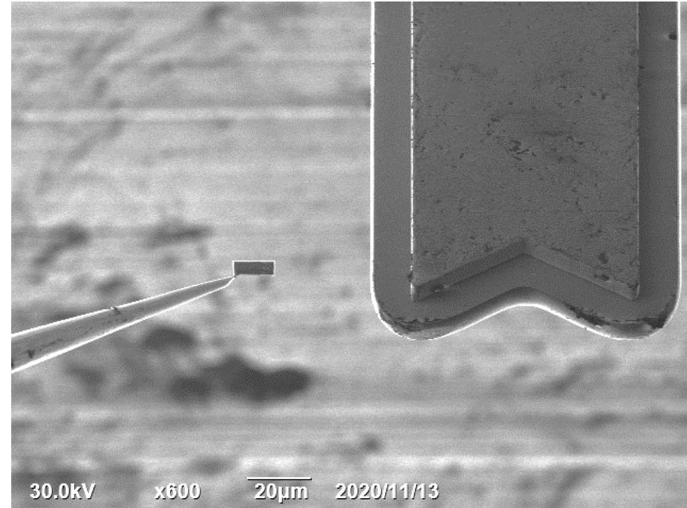
**ix) Omniprobe approach to TEM half-grid (Cu)**
