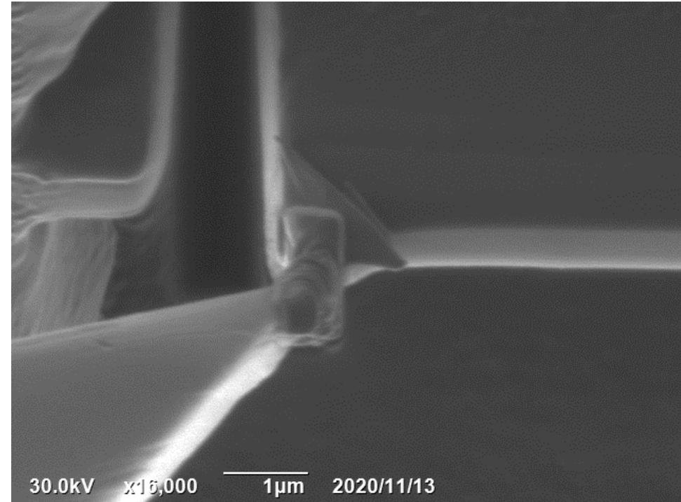
vi) Weld Omniprobe to sample
