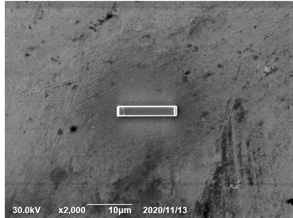
ii) Ion beam-assisted Pt deposition (Pt dep)
