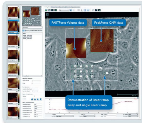
MIROView GUI enables seamless mode switching and automated measurements of multiple data types.
