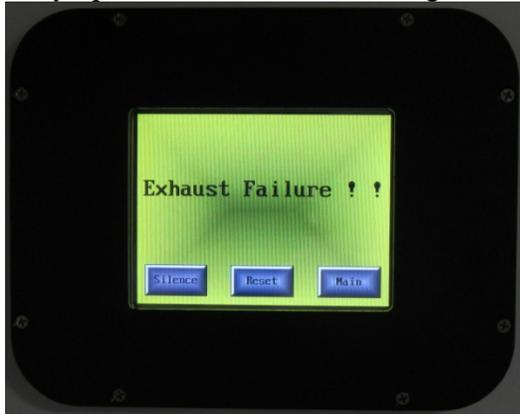
**Figure 13: Do not operate if an exhaust failure is indicated on the tool display!**
